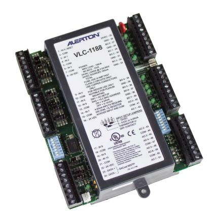
The Alerton® BACtalk® VLC-1188 is a versatile, fully programmable logic controller designed for central plant systems, air handling units, clean rooms, fume hoods, large terminal units, and similar control and process equipment. As a native BACnet controller, it integrates seamlessly with your BACnet system, communicating on a BACnet MS/TP LAN at up to 76.8 Kbps.
