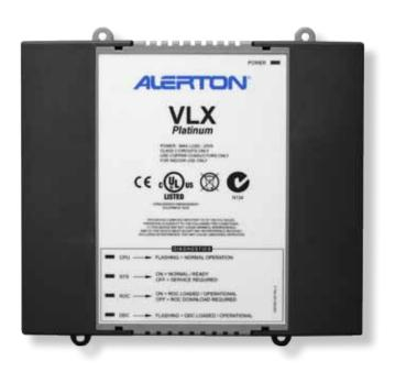
The Alerton® VLX-PLATINUM is a management-level controller that offers more than triple the memory of the current VLX controller to accommodate more BACnet objects such as alarms, schedules and trendlogs as well as more room for DDC. With an increased processor performance, this controller also offers significantly improved DDC execution speed.
