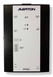
The Alerton® Integration Engine A-7 is a compact, embedded controller/server platform that combines integrated control, supervision, data logging, alarming, scheduling and network management functions with Internet connectivity and web-serving capabilities in a small, compact platform. The A-7 enables you to control and manage external devices over the Internet and view real-time information in web-based graphical displays.
