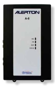
The Alerton® Integration Engine A-6 is a compact, embedded controller/server platform that combines integrated control, supervision, data logging, alarming, scheduling and network management functions with Internet connectivity and web-serving capabilities in a small, compact platform. The A-6 enables you to control and manage external devices over the Internet and view real-time information in web-based graphical displays.
