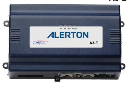
Alerton's Integration Engine A3-E is a compact, embedded controller/server platform. It combines integrated control, supervision, data logging, alarming, scheduling and network management functions with Internet connectivity and web serving capabilities in a small, compact platform. The A3-E makes it possible to control and manage external devices over the Internet and present real time information to users in web-based graphical views.
